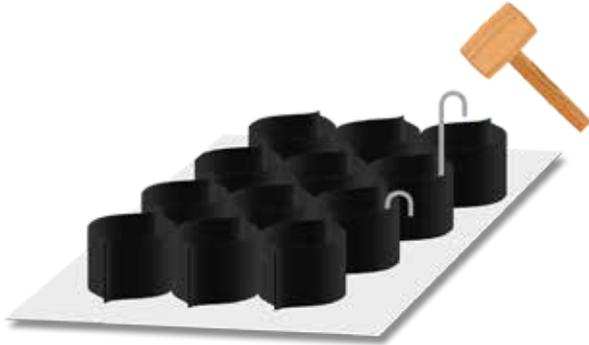
Ideally, when expanded the cells should be symmetrical and not distorted in any direction.
