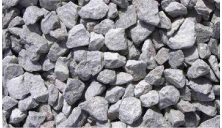
Typical examples of suitable clean angular gravel.
